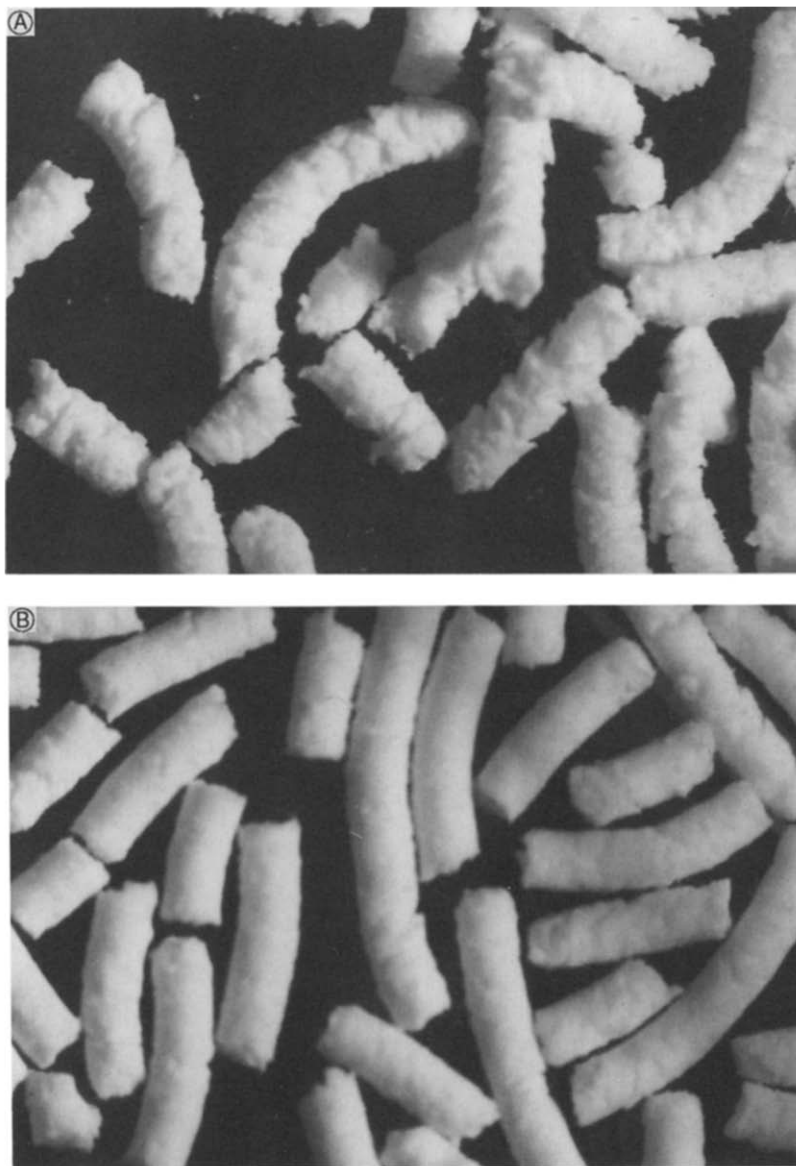
Fig. 6. Photographs of extrudate containing DCP/Avicel ® PH101/water (150:380:470 (w/w)). (A) Extrudate produced with an L/R ratio of 2 screen, (B) extrudate produced with an L/R ratio of 4 screen.
